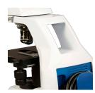
**INTEGRAL CARRYING HANDLE** Allows for one handed transportation of the microscope.
