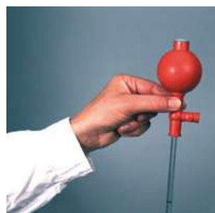
2. Intake by pressing on point B ↻
